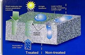
Silicone-based masonry water repellents provide the most effective protection against moisture decay. It will penetrate and provide water repellency(hydroxy groups) by chemically reacting with the substrates surface. These hydroxy groups will bond with the substrate and itself to produce a hydrophobic silicone resin network that inhibits water absorption into the substrate.
